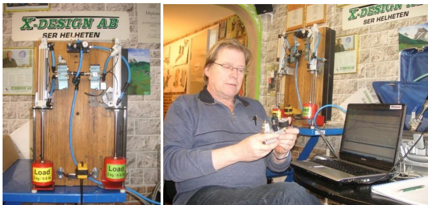
Picture shows parts of Per-Åke's testing system close up. The testing system consists of a compressor, tubing, computer with a special program for measurements and in the background the testing set-up. In his hand Per-Åke has a slightly larger X-Block than that installed at SCA. This Block has been especially designed for a customer in the USA.
